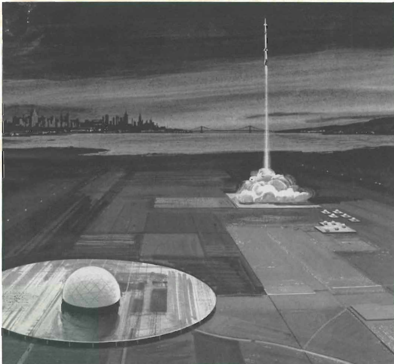
More than 450,000 pounds of thrust lifts the U. S. Army's Nike Zeus missile skyward in a cloud of vapor. The Nike Zeus missile being developed for the project by the Douglas Aircraft Company will be designed to intercept ballistic missiles traveling over 15,000 miles per hour, and destroy them at a safe distance from the defended area.
