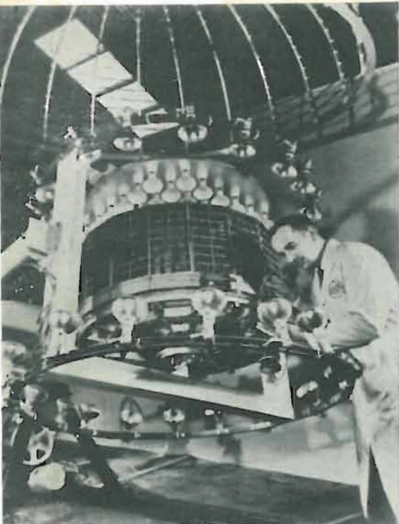
Fig. 2. The U.S. weather-eye satellite, "Tiros," was equipped with more than 9000 silicon solar cells. This represents one of the largest arrays of solar cells launched into orbit. In the illustration, a technician is taking measurements of the output of the solar cells prior to the launching of the weather satellite.
